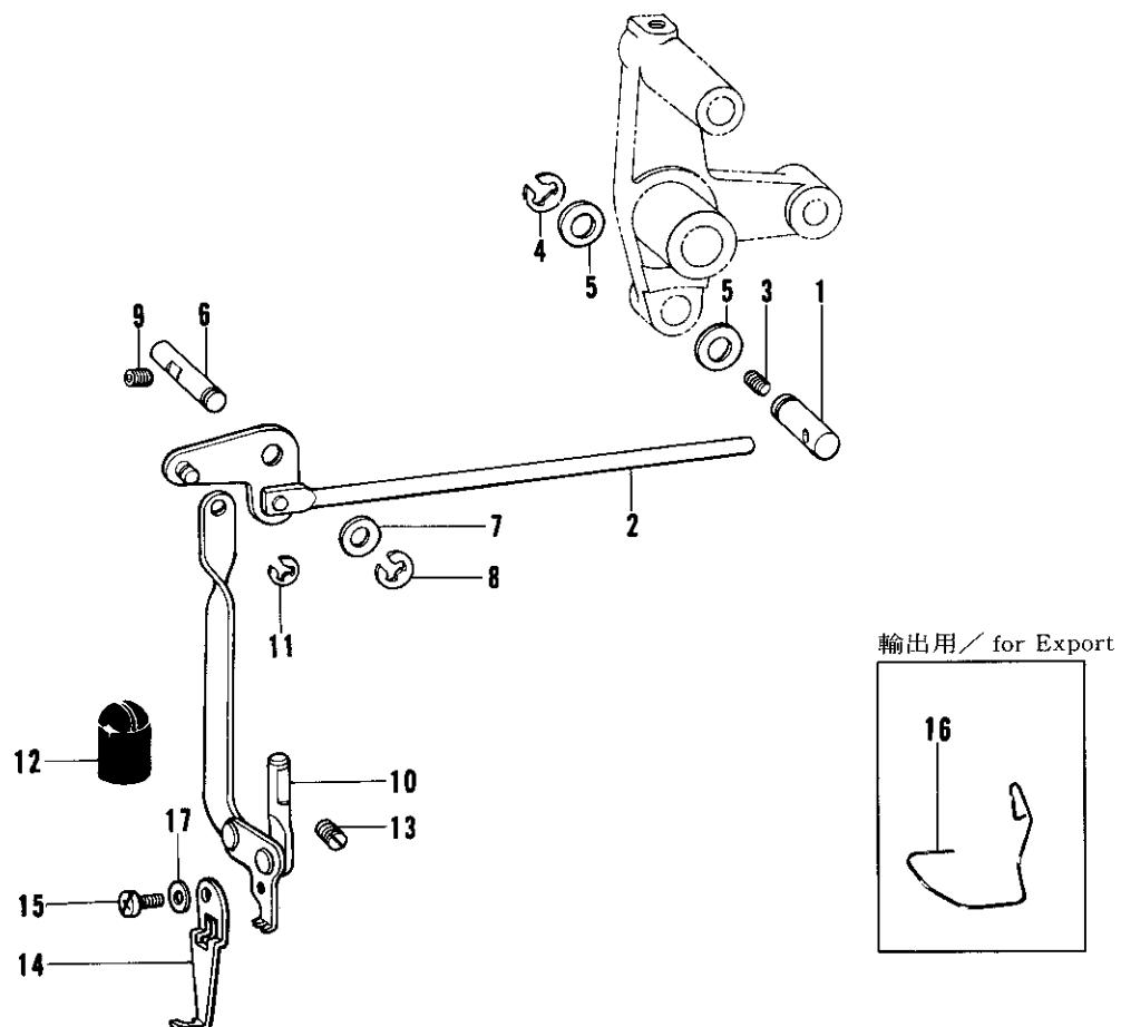
Q. 糸締め関係 / Thread nipper mechanism / Fadenspannvorrichtung
