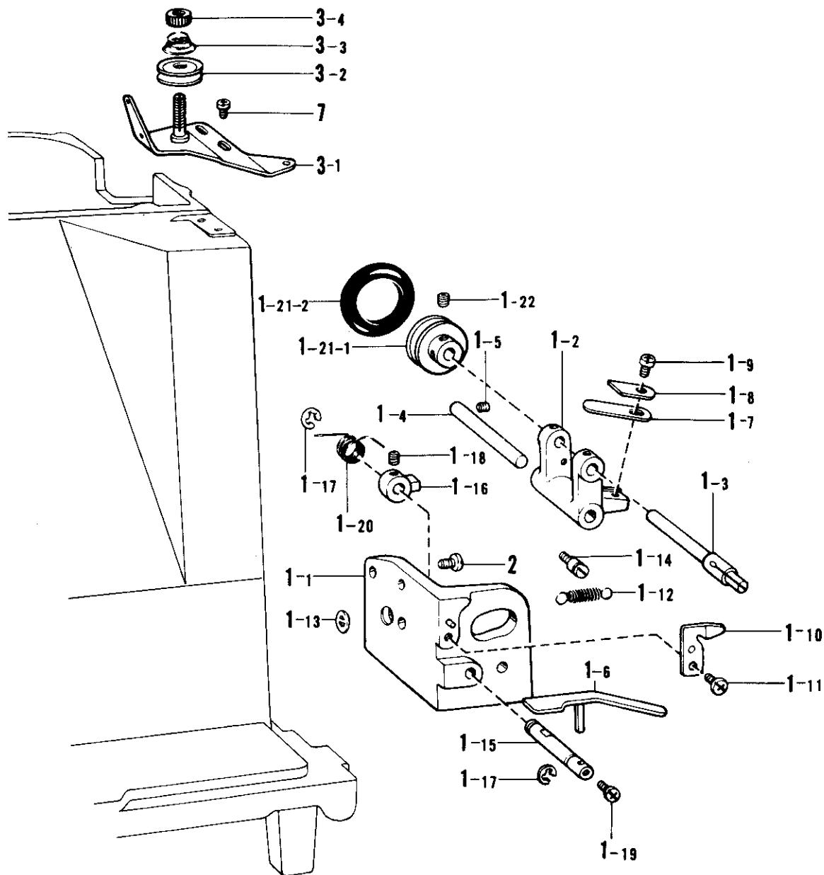
M. 糸巻き関係 / Bobbin winder mechanism / Spuler
